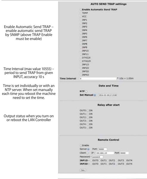
**Remote Control** - working as a server (receiving packets and enables / disables the corresponding output) or client (send packets to the server status change to INP1D or INP2D). LK working as a server can be actuated from any number of clients, provided it is set to the same password. Change in INP1D or INP2D low can switch outputs selected in the state of "ON", return to enter the high state output switches to "OFF".
