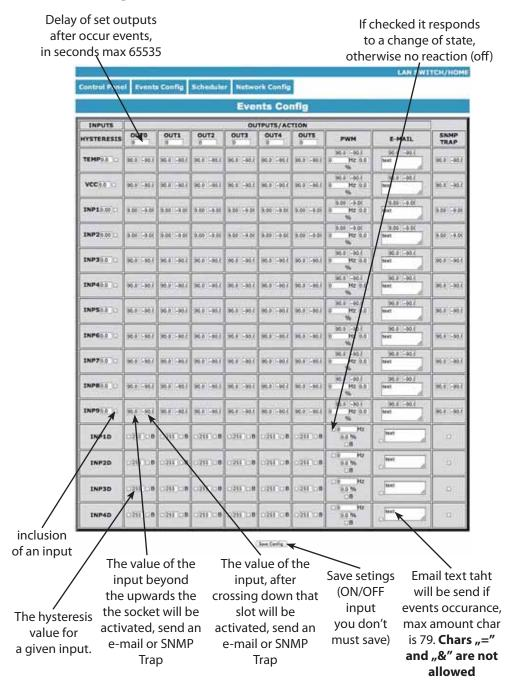
For logical input INP1D  $\div$  INP4D, e-mail and SNMP Trap notification are send when input level change from 1 to 0 or 0 to 1, additional to email text (at end) will be add value 1 or 0 mark actual input state.
